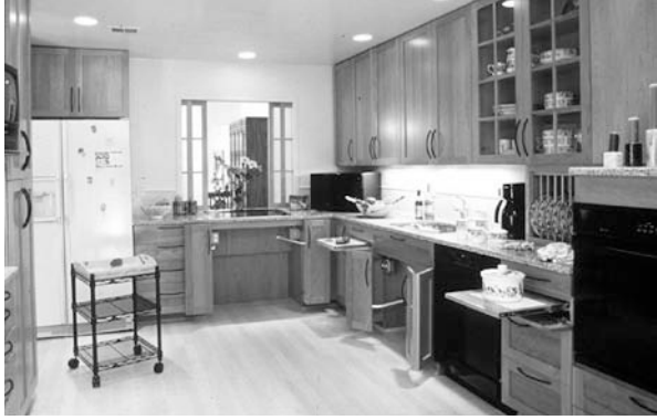
This kitchen provides ample work space, a raised dishwasher and lowered cooking surfaces.
